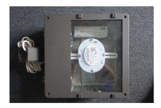
Retrofitting these type of fixtures are very easily accomplished. You just remove the bulb and reflector. A driver plate (not included) is mounted very easily to a screw port on the backside of the fixture. The light head is then screwed into the mogul base.
