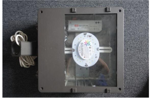
Retrofitting these type of fixtures are very easily accomplished. You just remove the bulb and reflector. A driver plate (not included) is mounted very easily to a screw port on the backside of the fixture. The light head is then screwed into the mogul base. You are able to adjust the light head to assist giving the proper lighting to the area. The light head can also be mounted on the backside of the fixture as shown in above photos.
